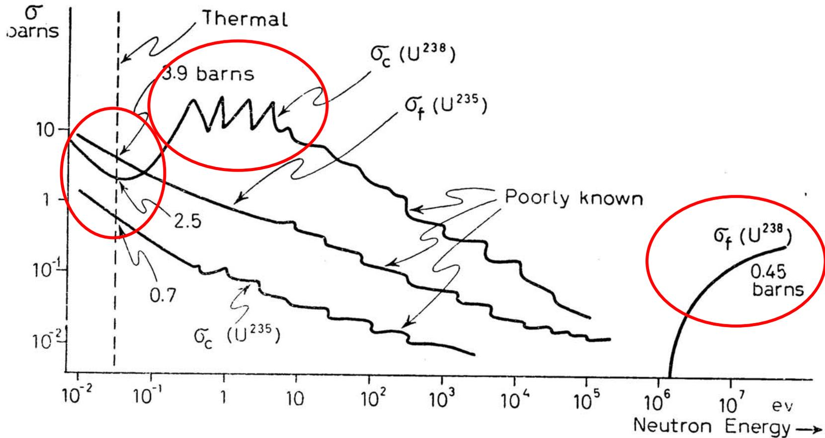
Fig. 77. - Uranium cross sections (separated isotopes).
